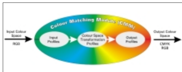
Figure 3 Color space transformation between device dependent color spaces and work color space over device profiles
